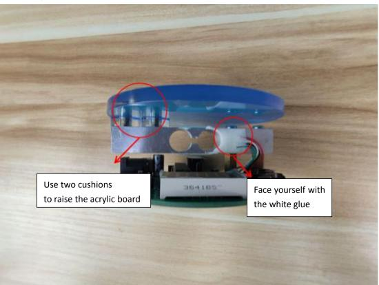
Finally, the acrylic film can be removed to become transparent;
